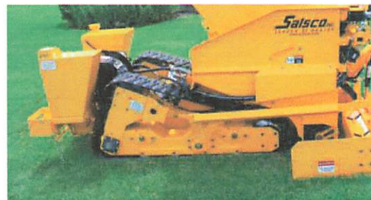
Tracks are fixed at 38" to accommodate screed style.
