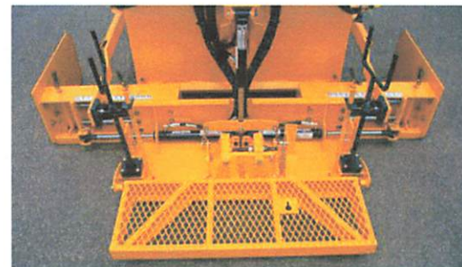
Hydraulic End-Gates move in & out, and have rulers on the top of the end gate to see where they are.
